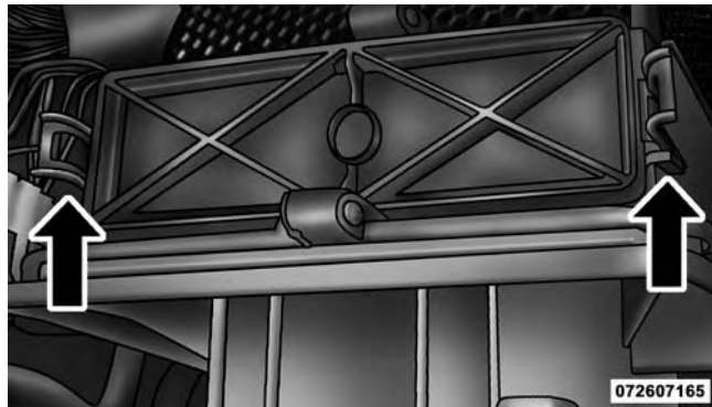
A/C Air Filter Replacement
