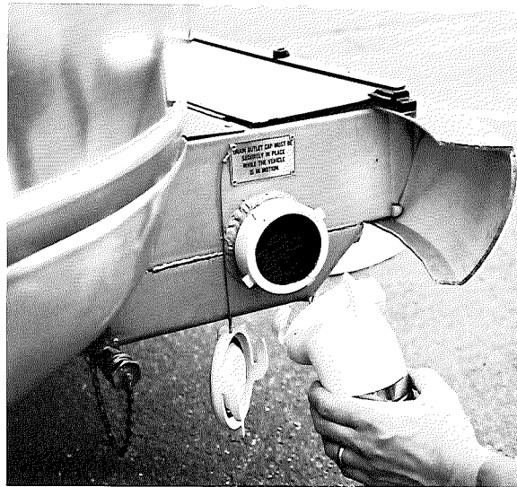
Rear Bath Sewage Outlet
