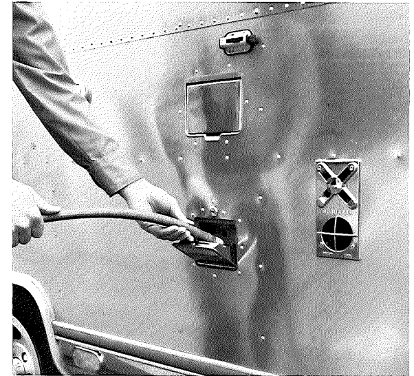
Water Tank Fill Spout
