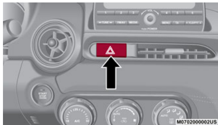
Hazard Warning Light Switch
