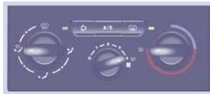
Air conditioning control panel
