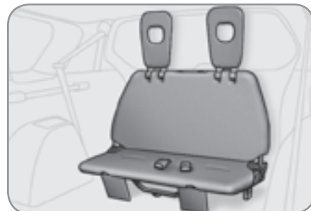
The rear bench seat can be folded. It retracts into a location in the floor of the vehicle.
