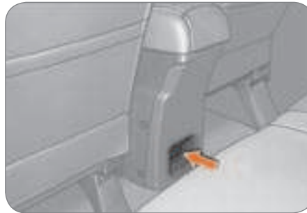
The three video sockets are located under the cover at the rear of the central armrest.
