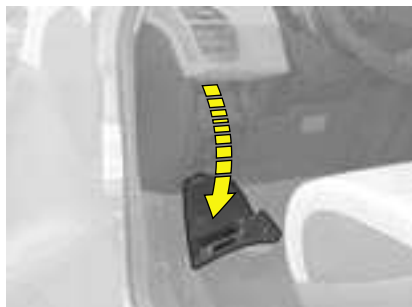
Access to the second glovebox fusebox
