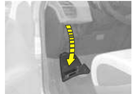
Access to the first glovebox fusebox
