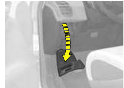
Access to the first dashboard fusebox
