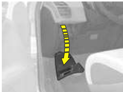
Access to the second dashboard fusebox
