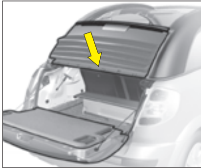
C. Open the rear screen by pressing on the control situated above the R in CITROËN.
