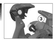
• Turn bulb holder **3** counterclockwise to remove it from the bulb housing.
