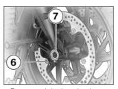
Remove right-hand axle clamping screw 6. with OF BMW Motorrad Integral ABS:
