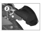
Pull the bulb housing to the rear until it is clear of holders 2.
