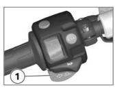
Press left-hand turn indicator button 1. The turn indicators are cancelled automatically after you have ridden for approximately 10 seconds, or covered a distance of about 200 m.◀
