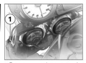
Remove securing screws 1 from both sides of the bulb housing.
