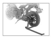
Press the lever down to the ground.
