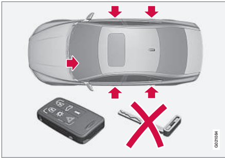
Locking/unlocking points with valet locking activated
