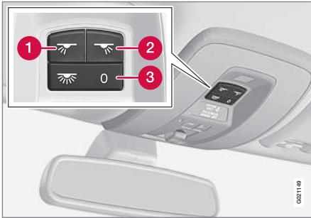
Light switches, front roof lighting
