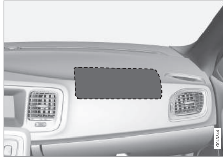
Location of the passenger's side front airbag
