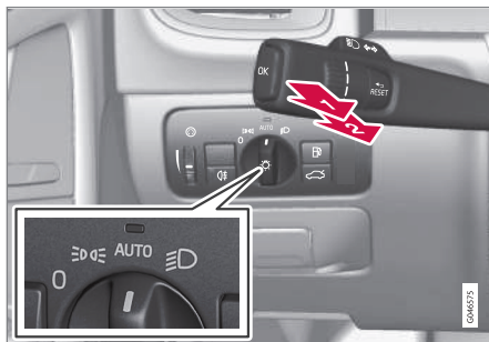
Headlight switch and steering wheel lever
