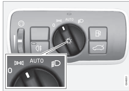
Headlight switch in the parking light position
