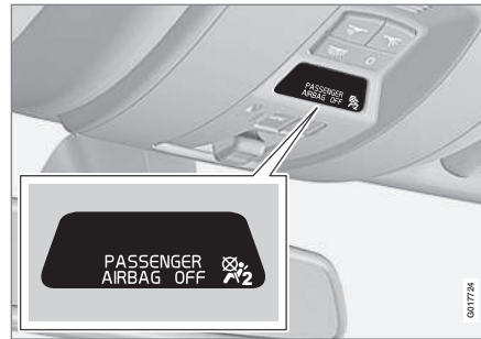
Occupant Weight Sensor (OWS) indicator light
