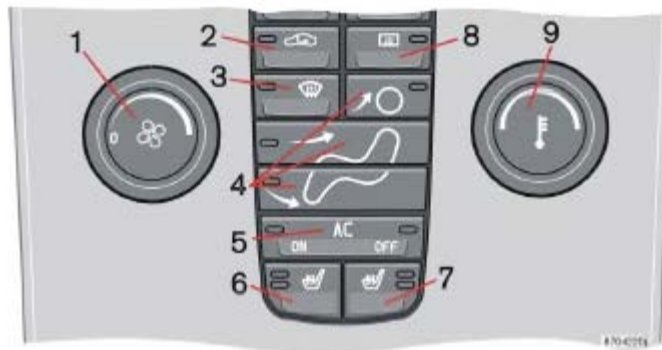
Climate system control panel
