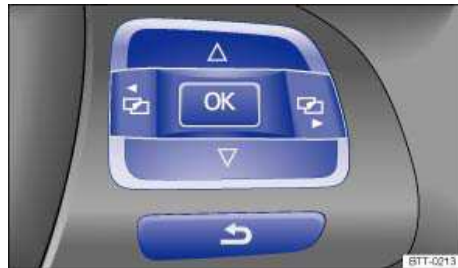
Fig. 13 Right side of the multi-function steering wheel: Controls for menus in the instrument cluster.
