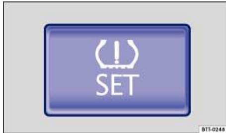
Fig. 96 In the glove compartment: SET button for the Tire Pressure Monitoring System.
