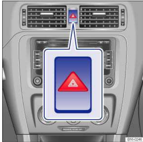
Fig. 152 In the center of the instrument panel: Button for the emergency flashers.
