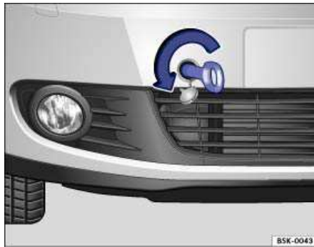
Fig. 191 In the right front bumper: Screwing in the towing eye.
