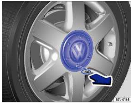
Fig. 164 Pulling the hubcap off.
