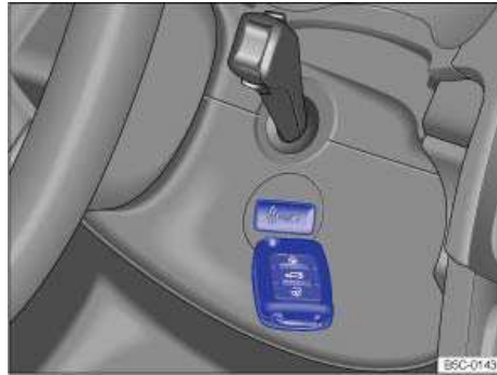
Fig. 114 Hold the remote control vehicle key to the right of the steering column: Emergency starting feature on vehicles with Keyless Access.
