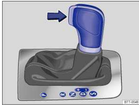
Fig. 116 Side view: Automatic transmission selector lever with shift lever release button (arrow).
