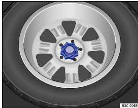
Fig. 93 In the luggage compartment: Handwheel holding the spare wheel in place.
