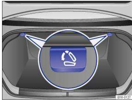
Fig. 85 On the left side of the luggage compartment: Release lever for the left-side rear seat backrest. The release lever for the right-side rear seat backrest is on the right side of the luggage compartment.
