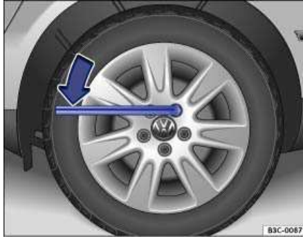
Fig. 168 Changing a wheel: Loosening wheel bolts.
