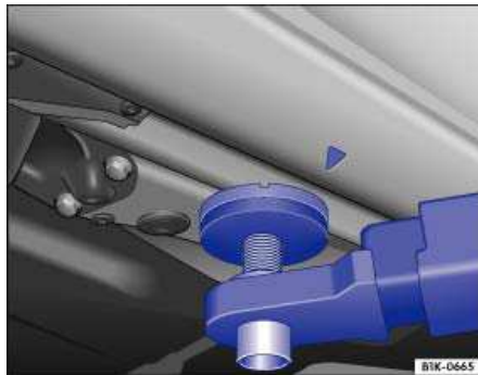
Fig. 151 Rear lift point for workshop hoist or floor jack.
