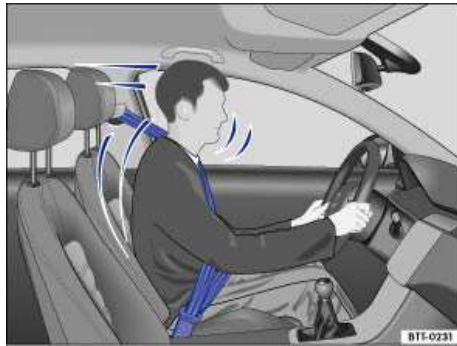
Fig. 49 Belted driver secured by the correctly worn safety belt in the event of a sudden braking maneuver.
