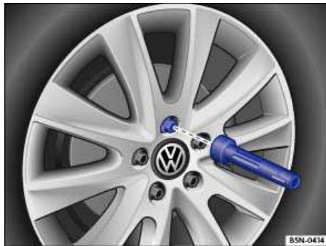
Fig. 171 Changing a wheel: Remove previously loosened wheel bolts using the screwdriver handle.
