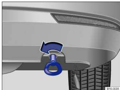
Fig. 193 In the rear right bumper: Screwing in the towing lug.
