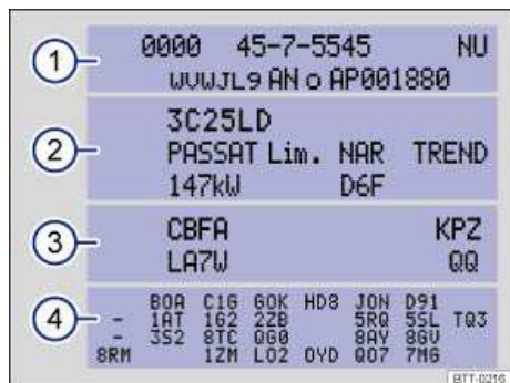
Fig. 14 Vehicle identification label: Shown in the example with engine identification code CBFA 3.
