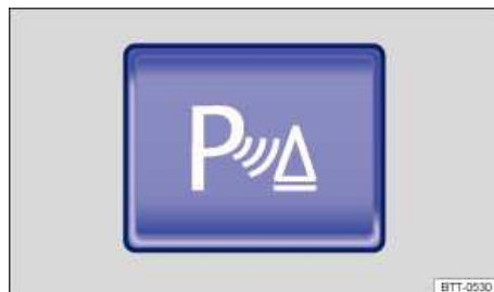
Fig. 143 In the center console: Button to switch the Park Distance Control system on or off.
