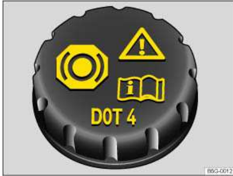
Fig. 133 In the engine compartment: Brake fluid reservoir cap (cap design may vary depending on vehicle equipment).
