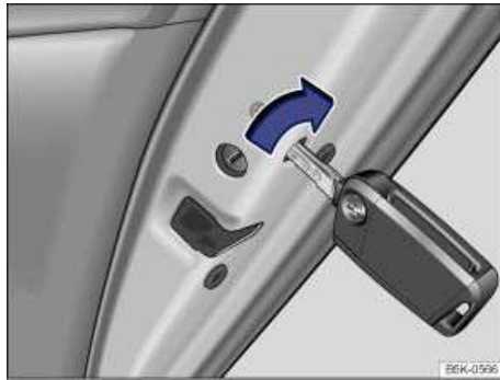
Fig. 166 On the front side of the right rear door: Locking the vehicle with the key bit in the vehicle key.
