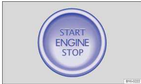
Fig. 122 In the lower center console: Starter button for the Keyless Access system.
