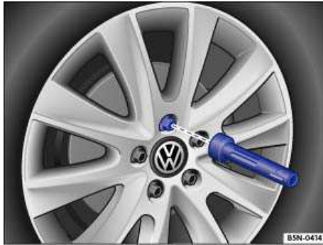
Fig. 181 Changing a wheel: Remove previously loosened wheel bolts using the screwdriver handle.
