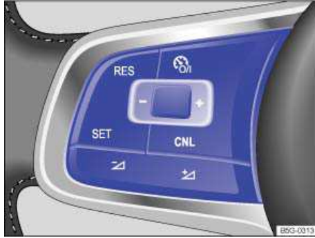
Fig. 137 Left-hand side of the multi-function steering wheel: Buttons for operating the cruise control .
