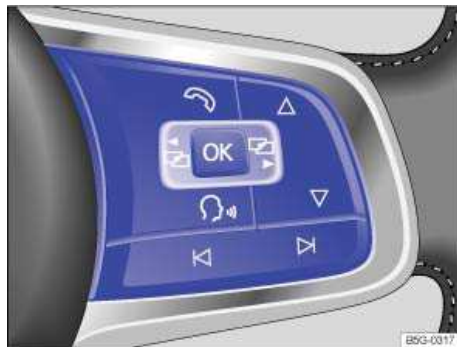
Fig. 13 Right side of the multi-function steering wheel: Controls for the menus and information displays in the instrument cluster.
