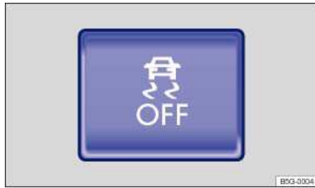
Fig. 132 In the center console: Button for switching ASR on and off manually.
