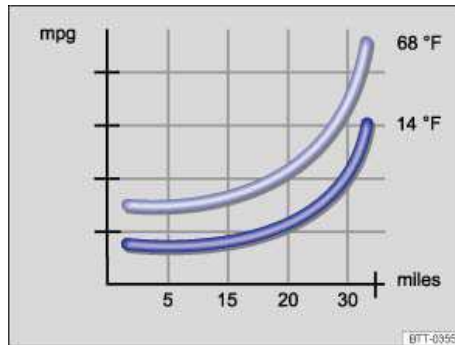
Fig. 134 Fuel consumption in miles per gallon (mpg) at 2 different outside air temperatures.
