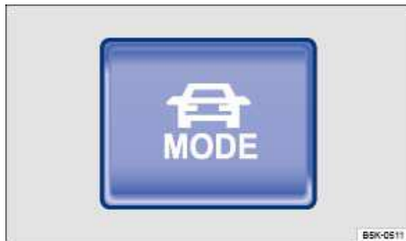
Fig. 146 In the lower section of the centre console: Driving Mode Selection button
