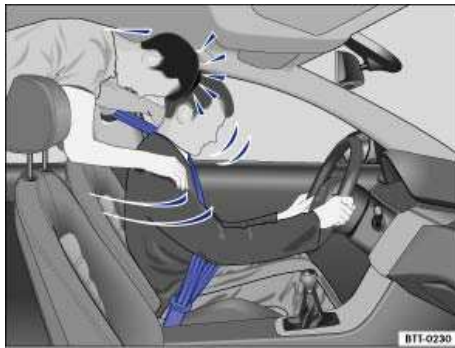
Fig. 50 Unbelted passengers in the rear seats are thrown forward on top of the belted driver.
