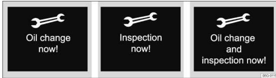
Fig. 11 In the instrument cluster display: Examples of service reminders when a service is due.
