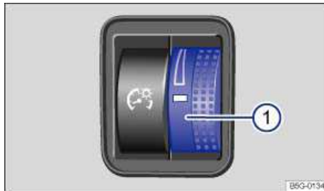
Fig. 76 To the left of the steering wheel: Thumbwheel to adjust instrument panel lighting 1.
