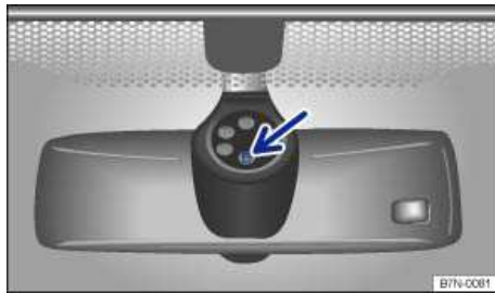
Fig. 83 Inside the front windshield above the inside mirror: Sensitive rain sensor surface.
