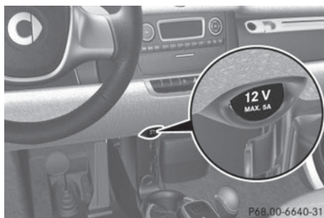
Auxiliary power outlet
