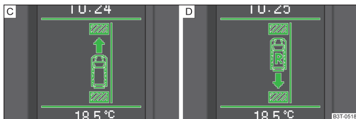
Fig. 104 Information display: Information to engage the forward gear C or the reverse gear D
