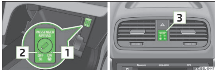
Fig. 127 Storage compartment: Switch for the front passenger airbag/indicator light for the deactivated front seat passenger airbag
