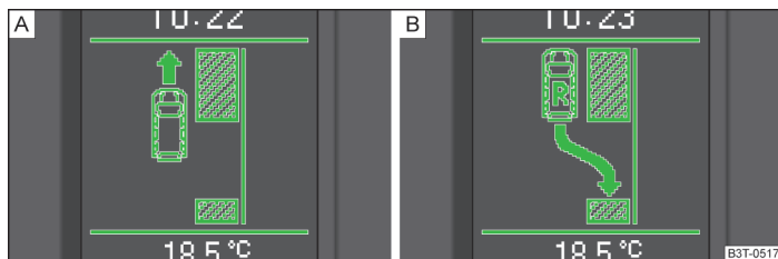
Fig. 103 Information display: Parking space detected including the information to continue driving A and to engage reverse gear B
