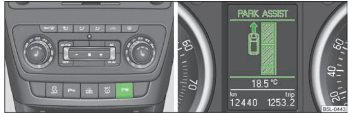
Fig. 102 Switch on display of the park assist in the information display/information display: Finding a suitable parking space
