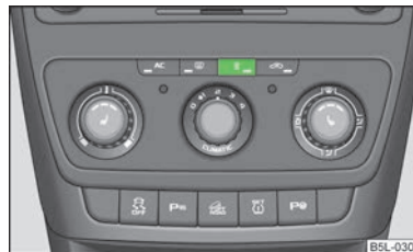
Fig. 92 Button for direct switching on/off of the auxiliary heating (auxiliary heating and ventilation) on the operating part of the air conditioning system
