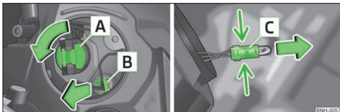
Fig. 128 Changing the bulb for main beam, separate daytime running lights, and parking light
