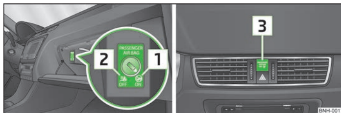
Fig. 86 Key-operated switch for the front passenger airbag/warning light for front seat passenger airbag deactivation
