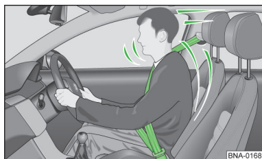
Fig. 21 Driver wearing a seat belt who is caught by the correctly fastened and adjusted seat belt in a sudden braking manoeuvre
