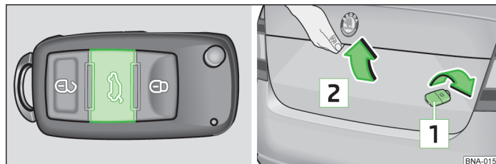
Fig. 11 Vehicle key with unlocking button for the boot lid / Opening the boot lid from the outside
