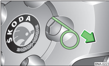
Fig. 77 Pulling off the caps from the wheel bolts
