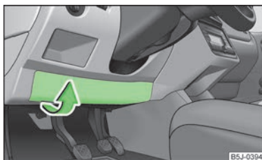
Fig. 142 Underside of the dash panel: Distribution board cover.
