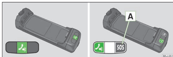
Fig. 94 Principle sketch: Adapter with one button/adapter with two buttons
