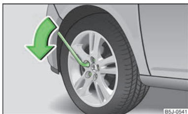
Fig. 133 Changing a wheel: Loosening the wheel bolts
