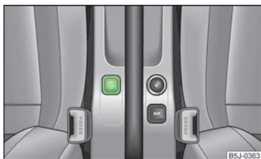
Fig. 130 Button for setting the tyre inflation pressure control value
