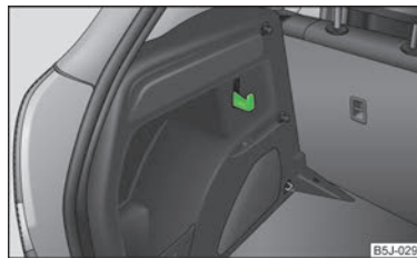
Fig. 45 Boot: folding hooks
