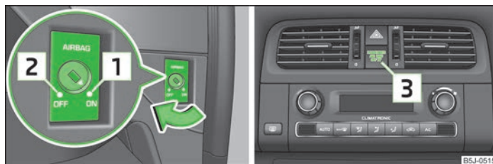
Fig. 106 Key-operated switch for the front passenger airbag/warning light for front seat passenger airbag deactivation
