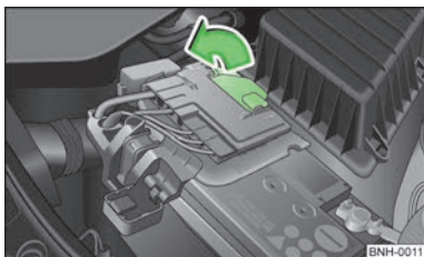
Fig. 123 Vehicle battery: Open up the cover
