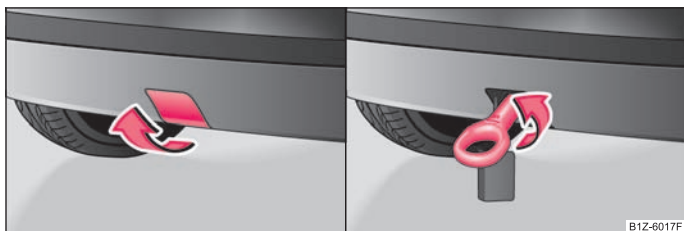
Fig. 142 Rear bumper: Removing the cover/installing the towing eye
