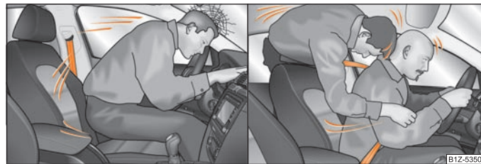
Fig. 91 The driver is thrown forward if not wearing a belt/the rear seat occupant is thrown forward if not wearing a belt
