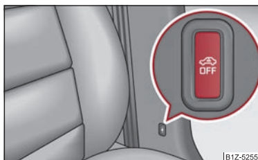
Fig. 31 Button for interior monitor and towing protection monitoring
