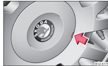
Fig. 136 Pulling off wheel trim cap on light alloy wheels
