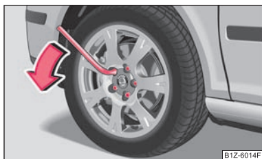
Fig. 137 Changing a wheel: Slackening wheel bolts
