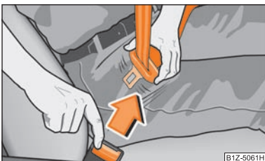
Fig. 94 Releasing lock tongue from belt lock
