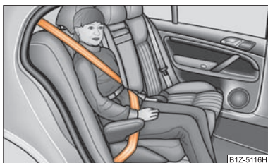
Fig. 108 Child seat in Group 3 installed on the rear seat facing the direction of travel
