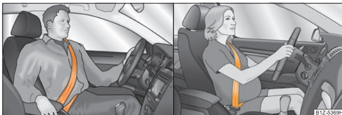
Fig. 92 Routing of webbing over the shoulders and the lap belt
