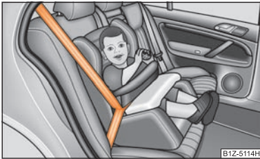
Fig. 106 Child seat with padded table in Group 1 installed on rear seat bench facing the direction of travel
