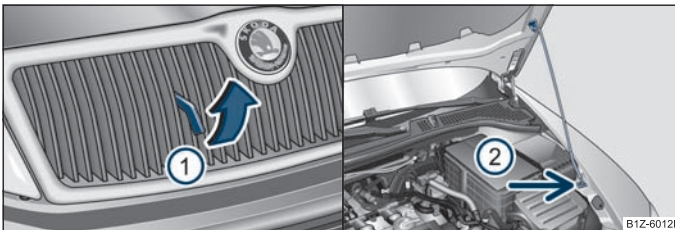
Fig. 121 Radiator grille: Release lever / securing the bonnet with the bonnet support
