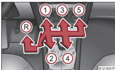
Fig. 85 The shift pattern: 5-speed manual gearbox
