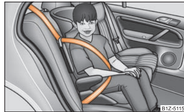
Fig. 107 Child seat in Group 2 installed on the rear seat facing the direction of travel
