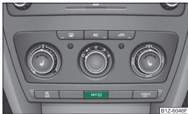
Fig. 113 Button for setting the tyre inflation pressure control value
