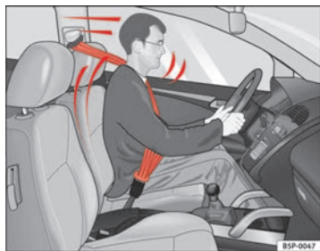
Fig. 10 A driver wearing the seat belt properly is secured by the belt in sharp braking
