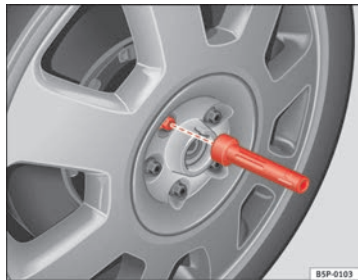
Fig. 139 Changing the wheel: Hexagonal socket in screwdriver handle to turn the wheel bolts
