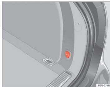
Fig. 136 Detailed view of the side trim in the luggage compartment: 12 volt socket
