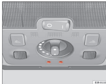
Fig. 95 Detail of headliner: ambient lighting
