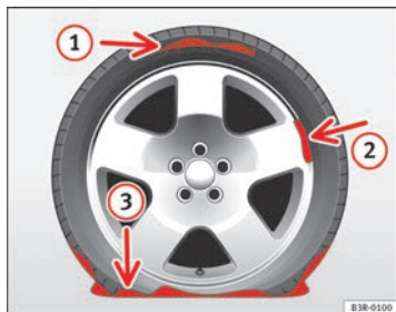
Fig. 198 The Tyre Mobility System is not suitable for repairing this type of damage to tyres.
