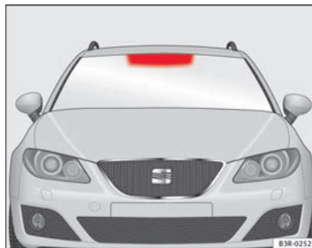
Fig. 173 Location of the electronic toll collection system
