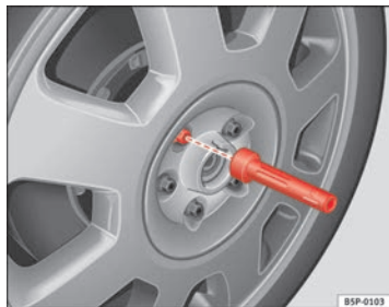
Fig. 196 Changing the wheel: Hexagonal socket in screwdriver handle to turn the wheel bolts
