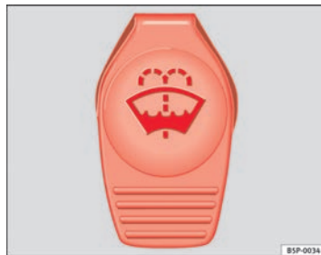
Fig. 180 In the engine compartment: Cap of windscreen washer fluid reservoir.
