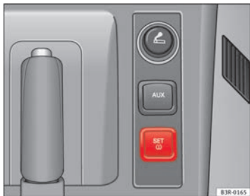
Fig. 186 Detailed view of the centre console: Button for the tyre pressure monitoring system
