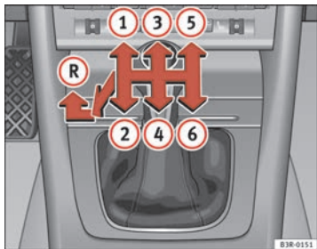
Fig. 153 Detailed view of the centre console: gear shift pattern of a 6-speed manual gearbox
