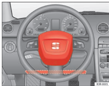
Fig. 17 Driver airbag in the steering wheel and knee airbag in the dash panel
