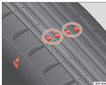
Fig. 174 Tyre tread wear indicators
