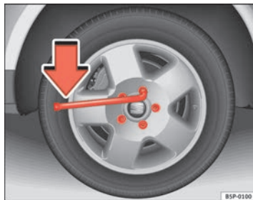
Fig. 178 Changing the wheel: loosen the wheel bolts
