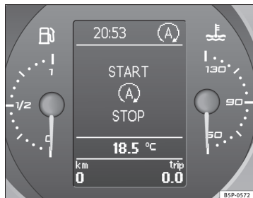
Fig. 142 Display on the instrument panel during Start-Stop function operation.
