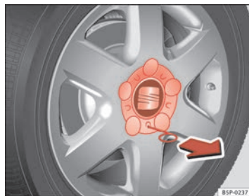
Fig. 177 Changing the wheel: Removing a hub cap
