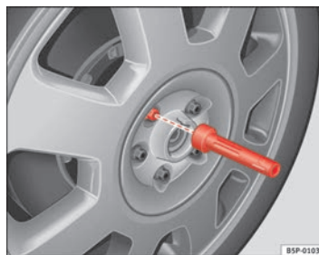
Fig. 182 Changing the wheel: Hexagonal socket in screwdriver handle to turn the wheel bolts
