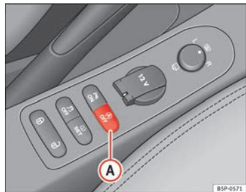
Fig. 139 The Start-Stop function button.
