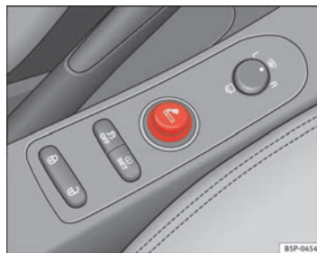
Fig. 117 The cigarette lighter is located in the electric socket on the front of the centre console
