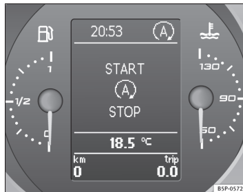
Fig. 140 Display on the dash panel during Start-Stop function operation.
