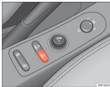
Fig. 50 Centre console: tyre monitor system button
