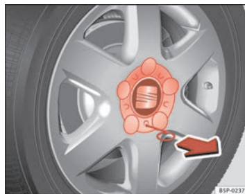
Fig. 176 Changing the wheel: Removing a hub cap
