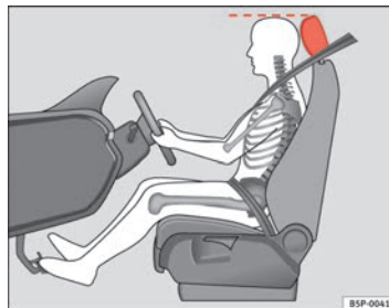
Fig. 2 Proper head restraint position for driver
