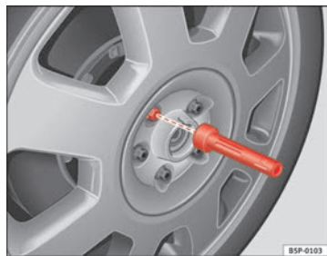
Fig. 180 Changing the wheel: Hexagonal socket in screwdriver handle to turn the wheel bolts
