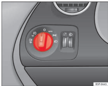
Fig. 73 Detailed view of dash panel: lights, fog light and rear fog light control
