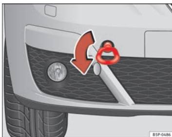
Fig. 205 The front right section of the vehicle: Fitting the front towing eye
