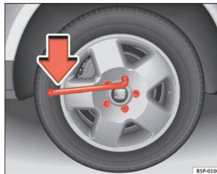
Fig. 171 Changing the wheel: loosen the wheel bolts
