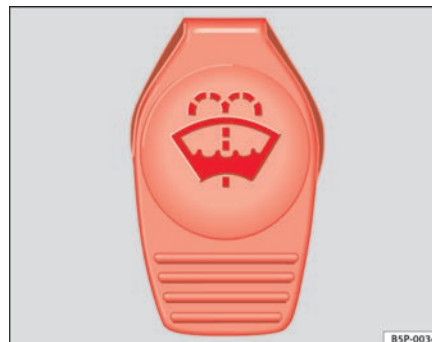
Fig. 161 In the engine compartment: Cap of windscreen washer fluid reservoir.
