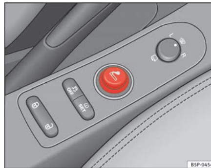
Fig. 117 The cigarette lighter is located in the electric socket on the front of the centre console
