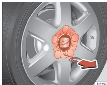
Fig. 170 Changing the wheel: Removing a hub cap
