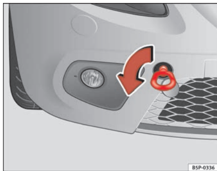
Fig. 199 The front right section of the vehicle: Fitting the front towing eye
