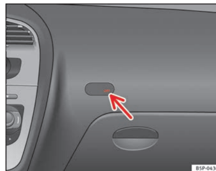
Fig. 27 Warning lamp for deactivated passenger airbag in centre console
