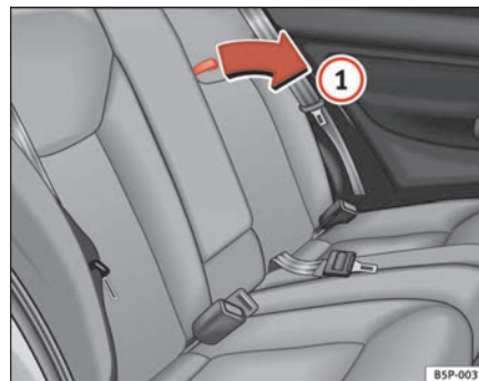
Fig. 109 Opening the rear drink holders
