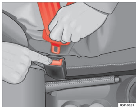
Fig. 16 Removing latch plate from buckle
