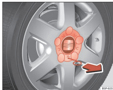
Fig. 169 Changing the wheel: Removing a hub cap
