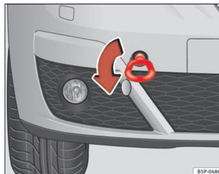
Fig. 198 The front right section of the vehicle: Fitting the front towing eye
