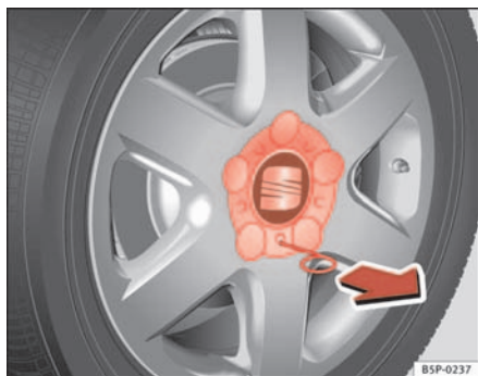
Fig. 129 Changing a wheel: Removing the wheel trim
