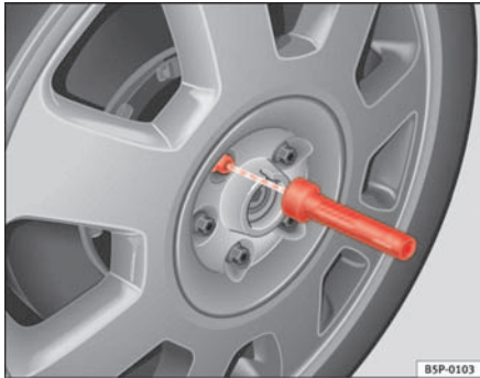
Fig. 134 Wheel change: Hexagon socket in screwdriver handle to turn the wheel bolts after they have been loosened
