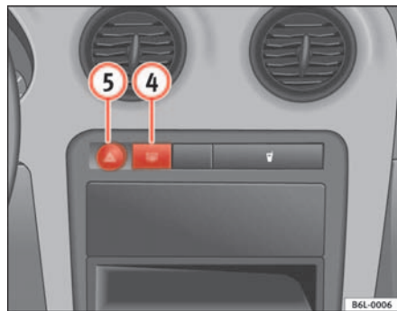
Fig. 59 Detail of the dash panel: Hazard warning light switch
