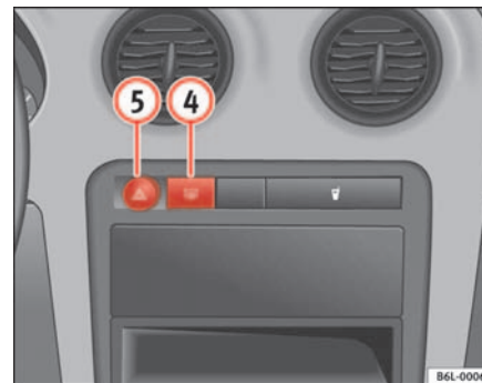
Fig. 58 Instrument panel: rear window heater switch
