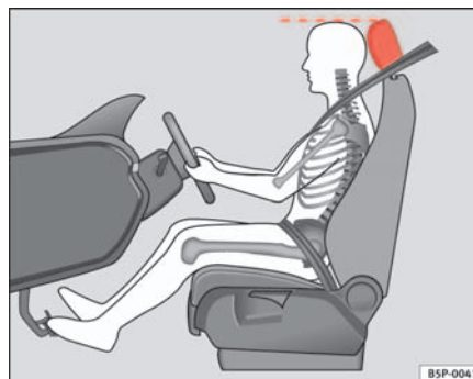
Fig. 2 Proper head restraint position for driver
