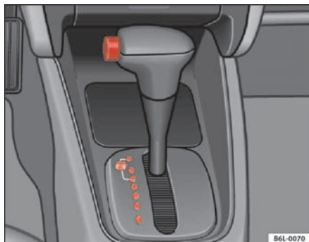
Fig. 95 Section of centre console: selector lever on cars with an automatic gearbox
