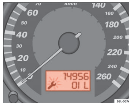
Fig. 39 Service interval display
