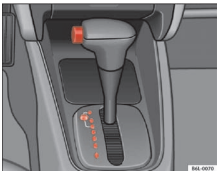
Fig. 94 Section of centre console: selector lever on cars with an automatic gearbox
