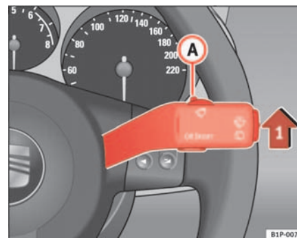
Fig. 65 Windscreen wiper lever
