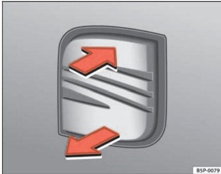
Fig. 50 Tailgate: Opening from the outside
