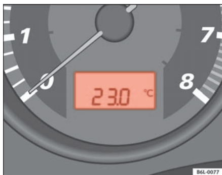
Fig. 36 Digital screen on the instrument panel: outside temperature display
