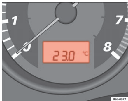
Fig. 38 Digital screen on the instrument panel: outside temperature display
