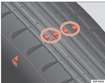
Fig. 127 Tyre tread wear indicators
