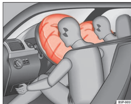
Fig. 19 Inflated front airbags
