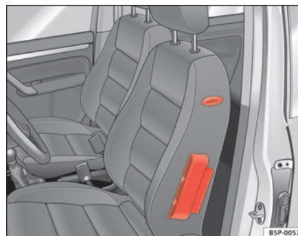
Fig. 21 Side airbag in driver seat
