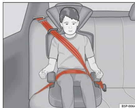
Fig. 29 Forward-facing child seat installed on rear seat.
