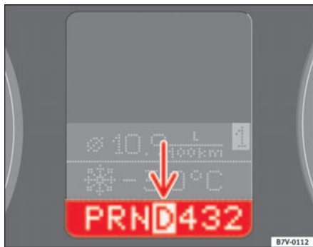
Fig. 129 Section of the instrument panel: display showing position of selector lever
