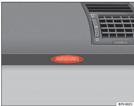
Fig. 23 Front passenger airbag located in dash panel
