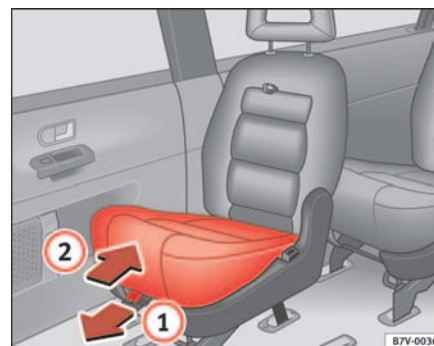
Fig. 40 Fitted child seat: raise the cushion
