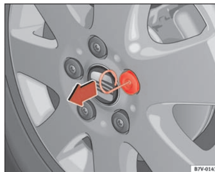
Fig. 157 Use the hook to pull off the cap
