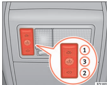
Fig. 67 Roof trim: switch for sliding/tilting roof
