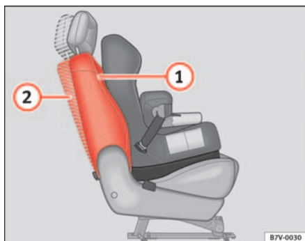
Fig. 34 Backrest adjustment when using ISOFIX child seats
