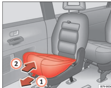
Fig. 41 Using the integrated child seat
