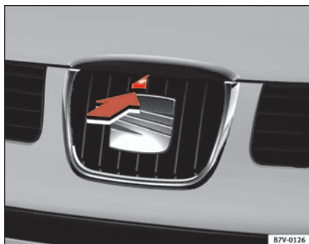
Fig. 140 Detail of the radiator grille: opening the bonnet
