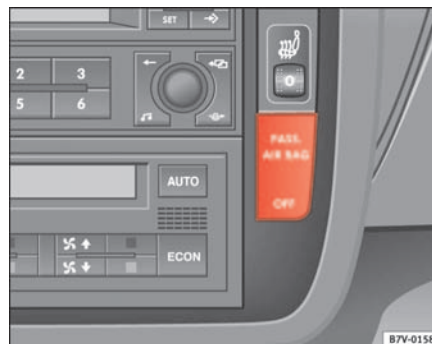
Fig. 29 Warning lamp for disabling airbag in dash panel
