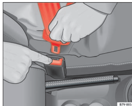
Fig. 16 Removing latch plate from buckle
