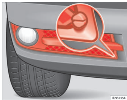
Fig. 173 Towing eye at the front of the vehicle
