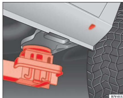
Fig. 176 Lifting with the lifting platform: lifting point at rear left
