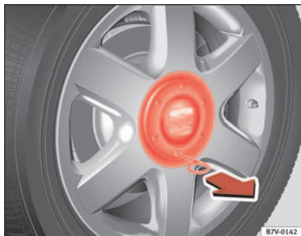
Fig. 156 Removing the hubcaps
