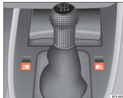
Fig. 66 Controls for electrically controlled vent wings
