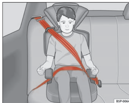
Fig. 32 Forward-facing child seat installed on rear seat.
