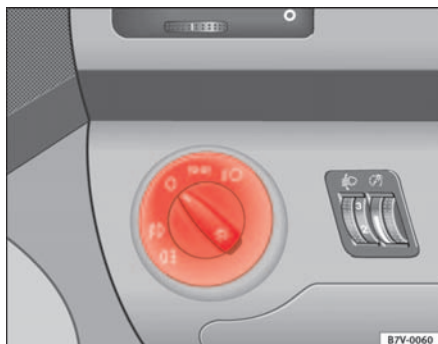
Fig. 71 Detail of the dash panel: Switch for lights, fog lights and rear fog light
