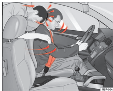
Fig. 8 The unbelted rear passenger is thrown forward violently, hitting the driver wearing a seat belt.
