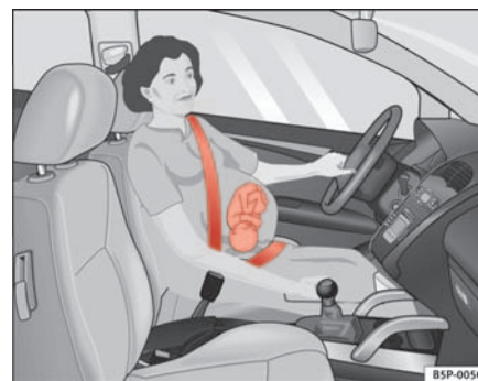
Fig. 14 Positioning seat belts during pregnancy
