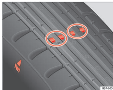
Fig. 150 Tyre tread wear indicators
