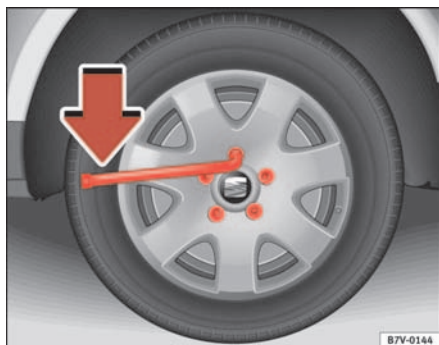
Fig. 158 Changing the wheel: Loosening the wheel bolts
