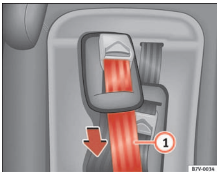
Fig. 38 Section of integrated child seat: Harness belt adjustment
