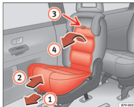
Fig. 35 Using the integrated child seat
