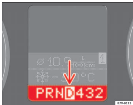
Fig. 131 Section of the instrument panel: display showing position of selector lever
