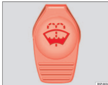
Fig. 145 In the engine compartment: Cap of windscreen washer fluid reservoir.
