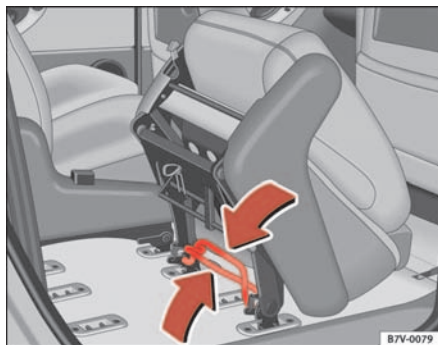
Fig. 93 Bar for removing and installing the individual seat
