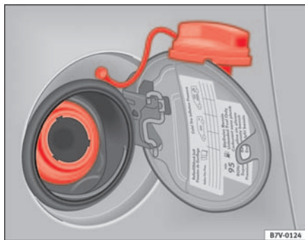
Fig. 138 Tank filler neck and tank flap
