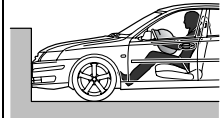
Sensors detect a deceleration and send a signal via the control module to a gas generator that inflates the airbag.
