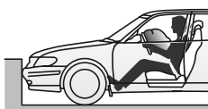
Sensor detects retardation and sends a signal via the control module to a gas generator that inflates the airbag.
