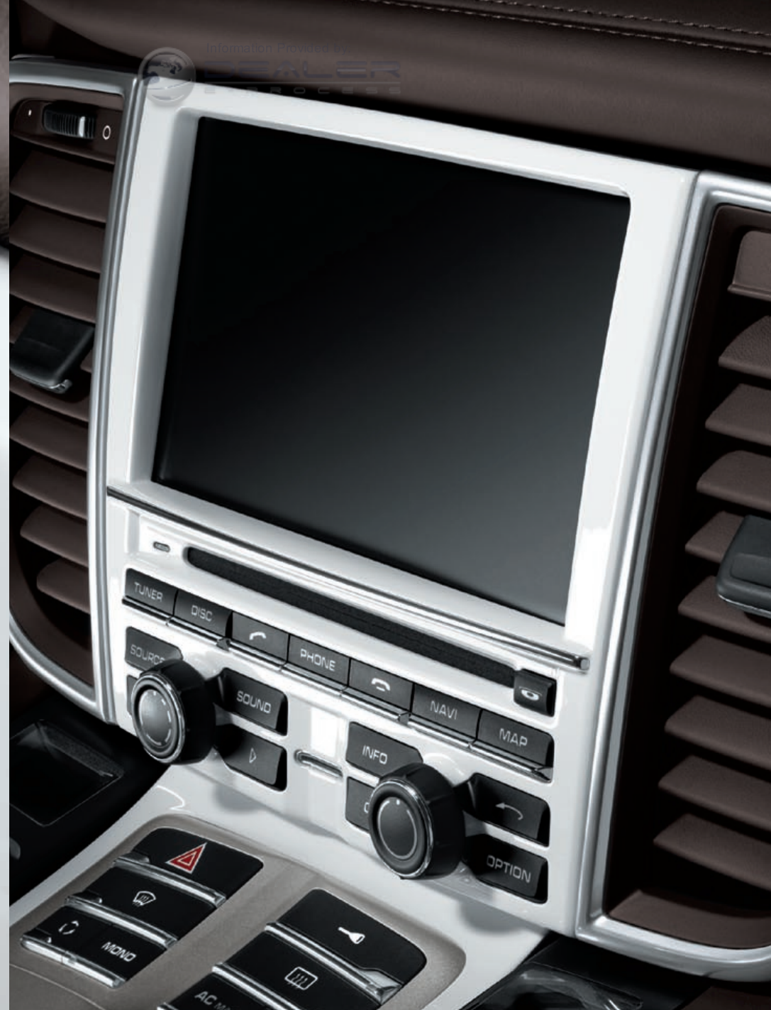
PCM surround painted
