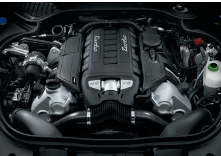
The twin-turbo V8 engine in the Panamera Turbo
