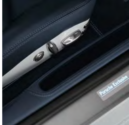
Inner door sill guards in leather, door sill guards with personalised logo in stainless steel, illuminated
