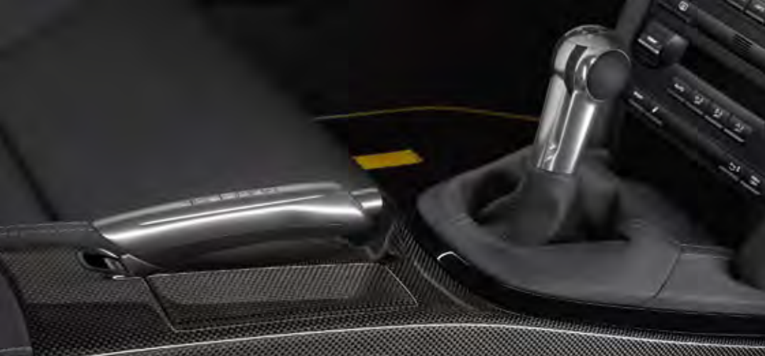
Gear and handbrake levers in aluminium I, rear centre console in carbon
