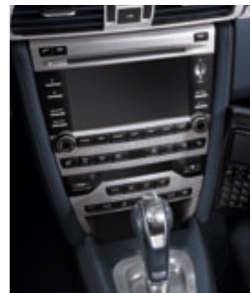
PCM package in Aluminium Look, PDK gear selector and handbrake lever in aluminium
