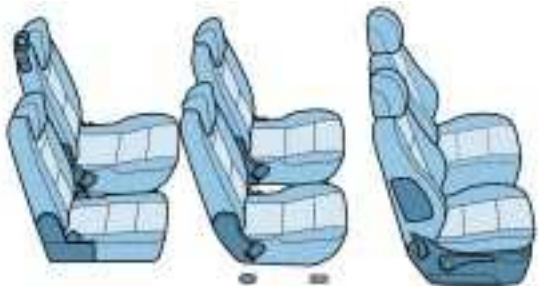
6 seats with an additional seat and the centre seat in the boot
