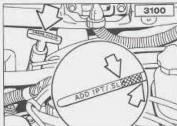
3100 V6: Checking Automatic Transaxle Fluid
