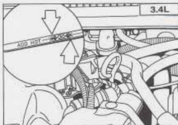
Twin Dual Cam 3.4L V6: Checking Automatic Transaxle Fluid
