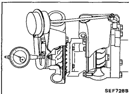
1. Inspect turbine and compressor wheel as follows:
