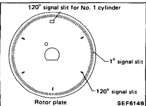
When the rotor plate passes the space between the L.E.D. and the Photo Diode, the slits of the rotor plate continually cut the light which is sent to the photo diode from the L.E.D. This causes generating rough-shaped pulses. They are then converted into on-off pulses by the wave forming circuit, which are sent to the E.C.U.
