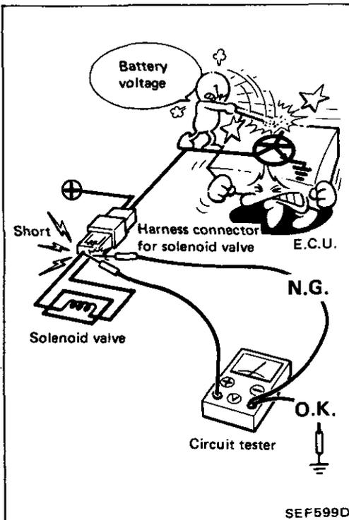
7. When measuring supply voltage of E.C.U. controlled components with a circuit tester, separate one tester probe from the other.
