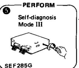
Perform self-diagnosis Mode III (for cylinder head temp. sensor).
