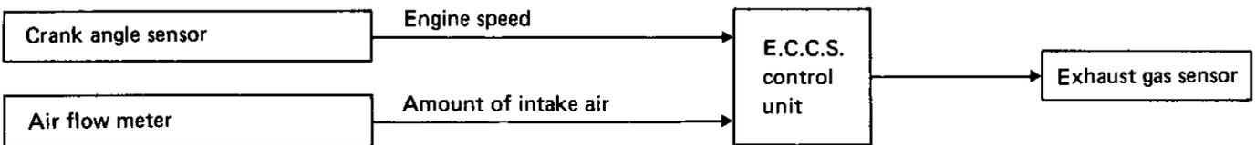
The E.C.U. controls the heater operation in the following way.
