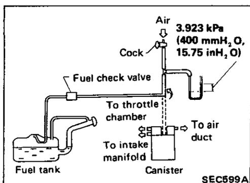
3. Connect a 3-way connector, a manometer and a cock (or an equivalent 3-way charge cock) to the end of the vent line.
