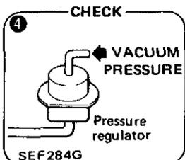
Apply vacuum/pressure to pressure regulator after disconnecting vacuum hose, and check idling.
