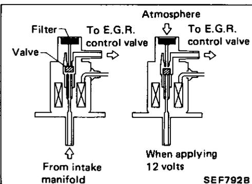
2. Check the solenoid valve for normal operation as shown.
