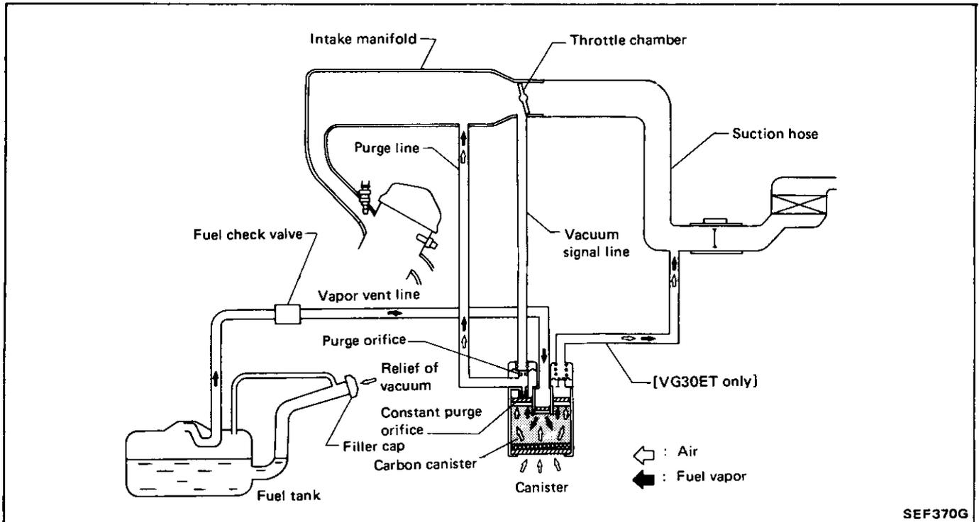
The evaporative emission control system is used to reduce hydrocarbons emitted to the atmosphere from the fuel system. This reduction of hydrocarbons is accomplished by activated charcoals in the carbon canister.
