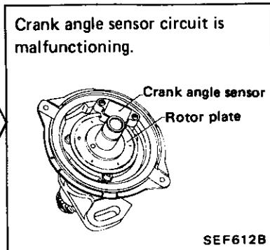
The 1° or 120° signal is momentarily missing, or, multiple, momentary noise signals enter.
