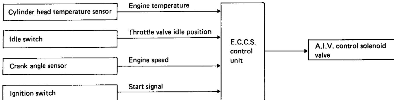
The air induction system is designed to send secondary air to the exhaust manifold, utilizing a vacuum caused by exhaust pulsation in the exhaust manifold.
