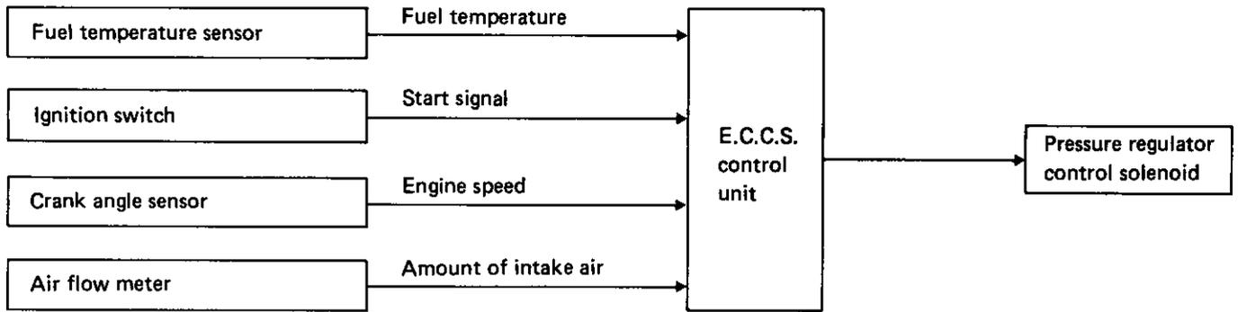
This system improves the startability in hot condition by cutting off the intake manifold vacuum and increasing the fuel pressure.
