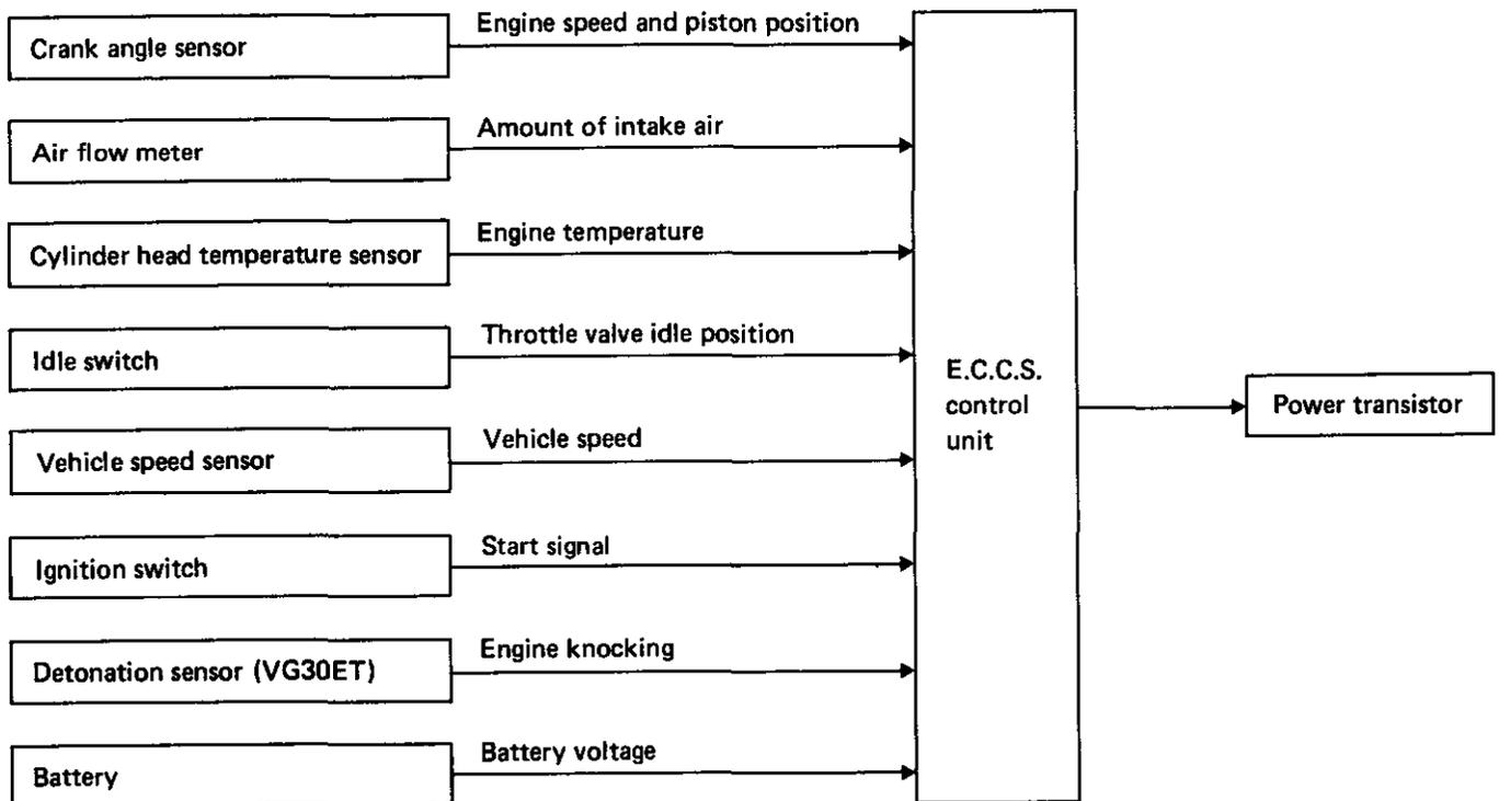
Ignition timing is controlled, corresponding to the engine operating conditions, by the E.C.U.: that is, as the optimum ignition timing in each driving condition has been pre-programmed in the control unit, the ignition timing is determined by electrical signals processed in the unit.
