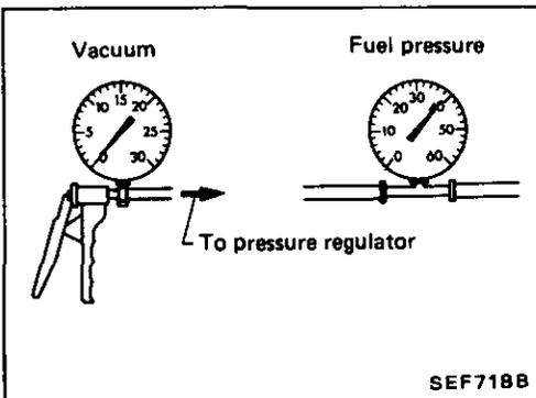
10. Turn ignition switch to "ON" and read the indication of fuel pressure gauge as vacuum is changed.
