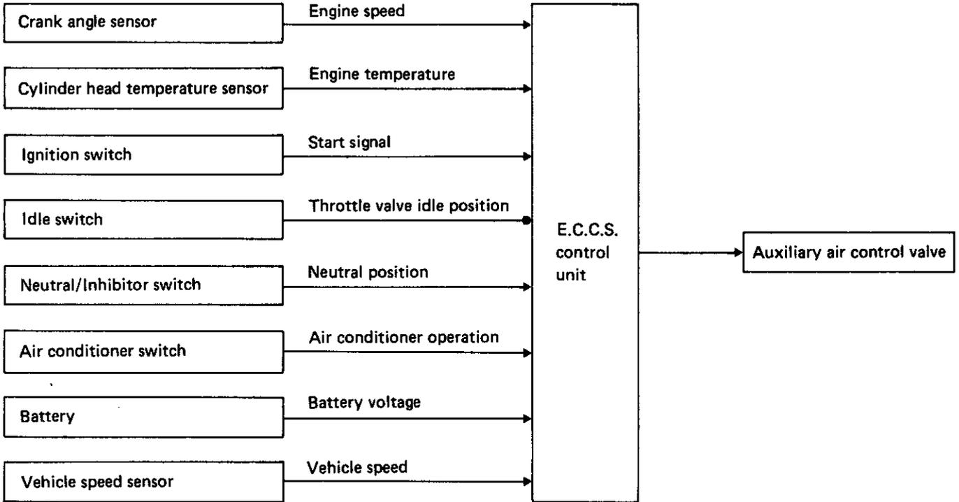
The idle speed is controlled by the E.C.U., corresponding to the engine operating conditions. The E.C.U. senses the engine condition and determines the best idle speed at each cylinder head
