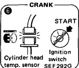
Start with cylinder head temp. sensor connector disconnected.
