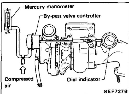
2. Check operation of by-pass valve controller.
