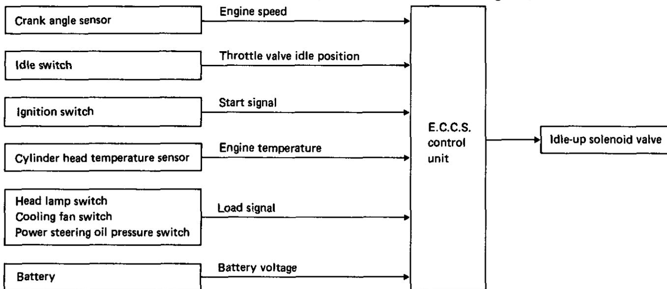
The idle speed is compensated by the E.C.U. to prevent rough idle when any of the following conditions are met.
