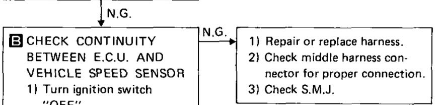
**B CHECK CONTINUITY BETWEEN E.C.U. AND VEHICLE SPEED SENSOR**
