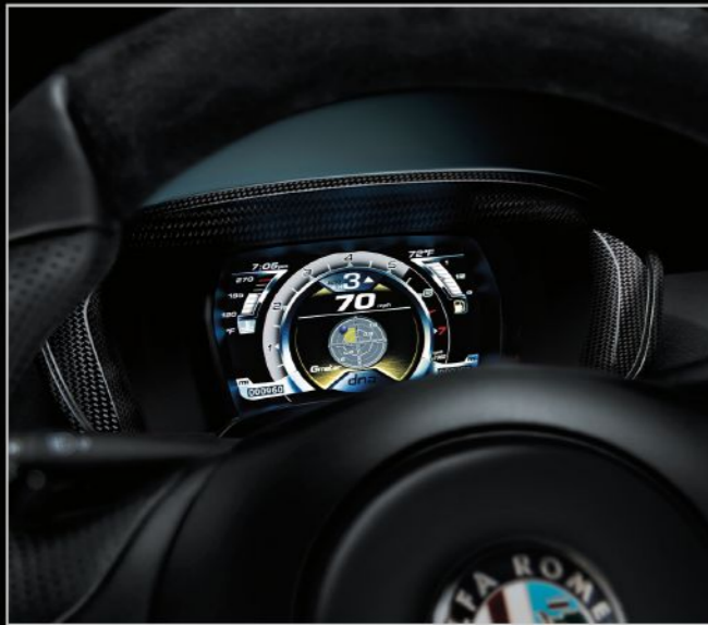
Full-digital instrument cluster with Thin Film Transistor (TFT) display and carbon fiber cluster surround
