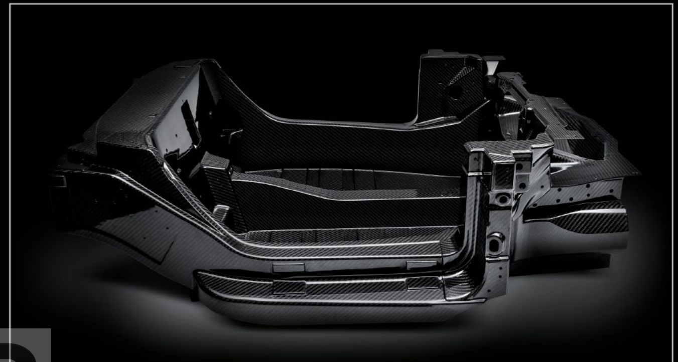
Genuine carbon fiber monocoque chassis
