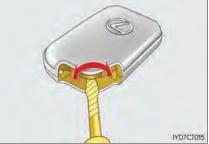
Remove the depleted battery. Insert a new battery with the "+" terminal facing up.
