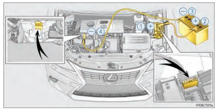
3 Connect the jumper cables according to the following procedure:
