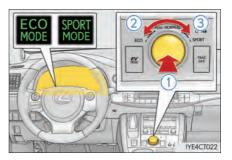
When the driving mode select switch is turned left, the "ECO MODE" indicator comes on in the instrument cluster.
