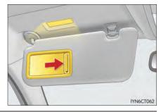
If the vanity light remain on when the power switch is turned off, the light will go off automatically after 20 minutes.
