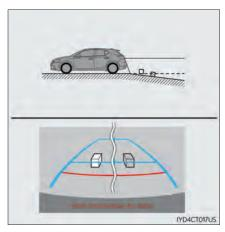
• When any part of the vehicle sags When any part of the vehicle sags due to the number of passengers or the distribution of the load, there is a margin of error between the fixation guide lines on the screen and the actual distance/ course on the road.
