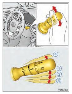
The sensor sensitivity can be adjusted when "AUTO" is selected.
