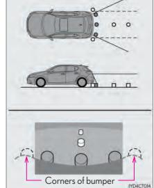
The camera for the rear view monitor system is located above the
