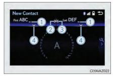
(4) When this indicator is shown, you can change to input mode by moving the controller backward.
