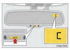
Drive the vehicle at 5 mph (8 km/h) or less in a circle until a direction is displayed.
