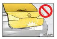
• Do not pull on the back door damper stay to close the back door, and do not hang on the back door damper stay.
