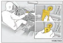
**3** Press the power switch within 10 seconds of the buzzer sounding, keeping the brake pedal depressed.
