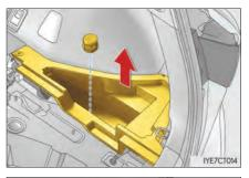
**4** Remove the 12-volt battery maintenance cover.
