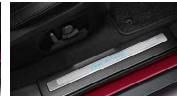
Personalized Sill Treadplates ‡ Personalized illuminated treadplates allow you to choose your own message using an approved set of fonts/typefaces which will be highlighted in White illumination when the front doors are open.
