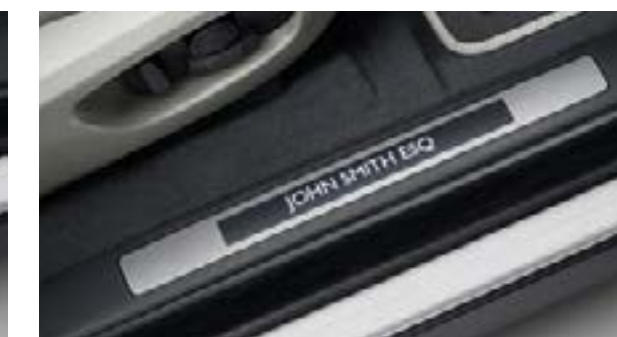
Sill Treadplates – Personalized VPLCS0343PVJ – Ebony VPLCS0343LAA – Lunar (not shown) Personalized illuminated treadplates allow you to choose a personalized message using an approved set of fonts/typefaces which will be highlighted in White illumination when the front doors are open. Available as front pair only.
