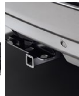
Tow-Hitch Receiver LR007482 Tow your boat or trailer with help from this sturdy, lockable hitch receiver. Handles up to 3,500lbs/1587.6kg trailer load capacity and a 330.0lbs/149.7kg tongue weight capacity.
