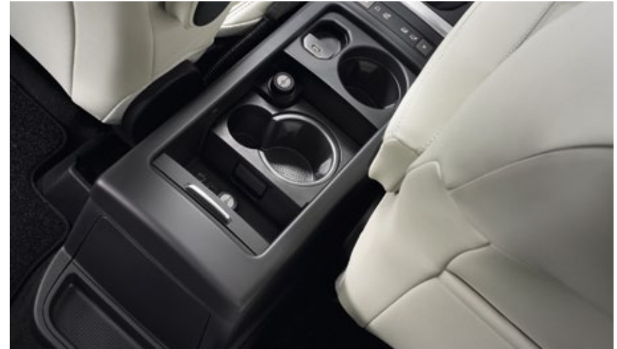
CENTER CONSOLE STORAGE. The rear of the center console features an additional storage box for small items, a 3.5mm auxiliary socket for MP3 players and a power socket, which can be used to recharge PCs and other low-wattage electrical equipment.
